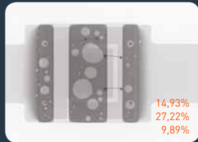
X-Ray capture of even acceptable (but not for LIVA Energy standard) thermal pad soldering
